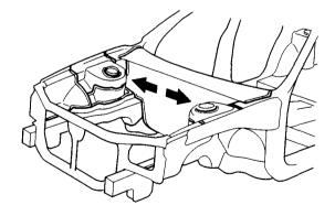
5. Apply sealer on any area that the replacement part will cover. Smooth the sealer with a brush if necessary.
