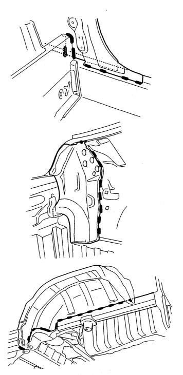
7. Tack weld the center pillar stiffener, and set the new rear fender panel.
