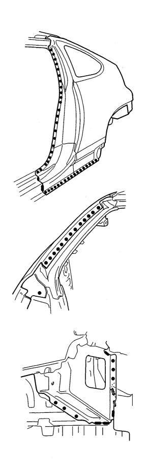
• Finish the joint of the rear fender panel with fillet weld, and grind the finishing allowance with a disc sander until it is smooth.
