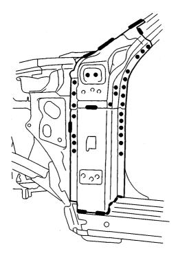
5. Tack weld the center pillar stiffener, and set the rear fender panel.
