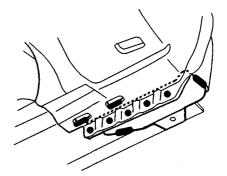
9. Weld the front side sill reinforcement.
