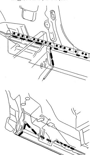
• Weld the side sill to the front inner lower pillar.
