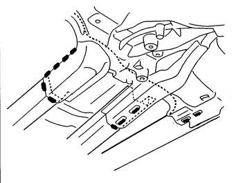
NOTE: When replacing the side sill, weld the garage jack base and side sill of the new part.
