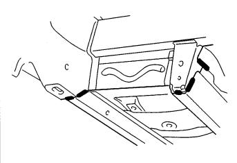
• Weld the tunnel frame extension, front side outrigger, and side sill.
