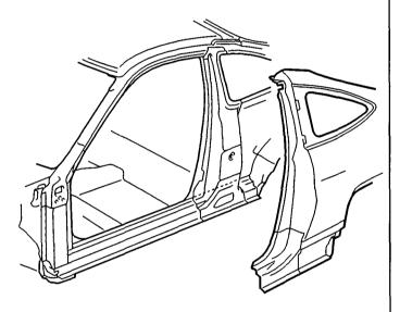
4. Remove the rear fender panel and center pillar stiffener, and main weld the front floor, side sill, front lower pillar, and front pillar lower stiffener.
