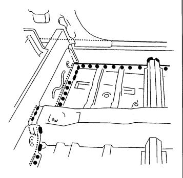
• Weld the front floor frame and tunnel frame of the front floor to the rear frame outrigger and middle crossmember frame.
