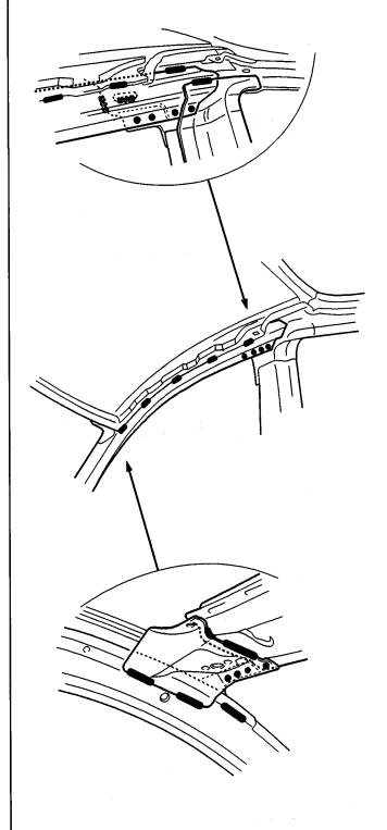
Weld the front roof rail reinforcement.
