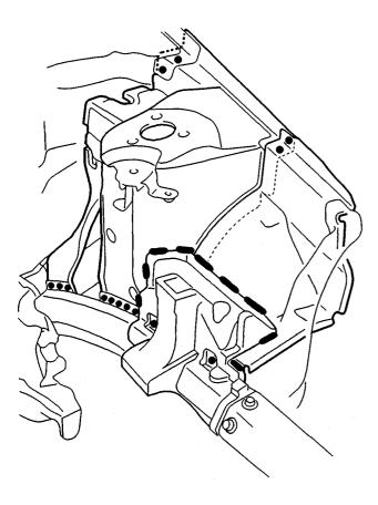
From passenger compartment side, plug weld the holes in the dashboard lower, wheelhouse B and damper base.
