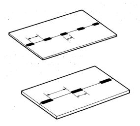
• The thinner the sheet or plate, the shorter the tack welding pitch and bead.
