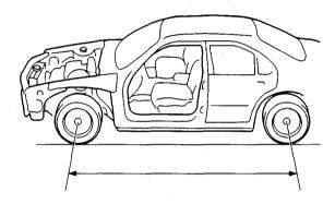
• If there is any twisting to the body, measure with a frame centering gauge.
