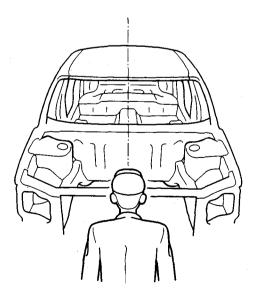
• To measure body dimensions, use a universal tram gauge and convex tool.
