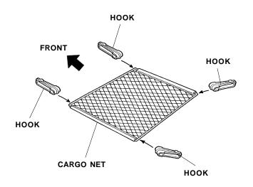
Attach the hooks you just installed to the anchors in the trunk.
