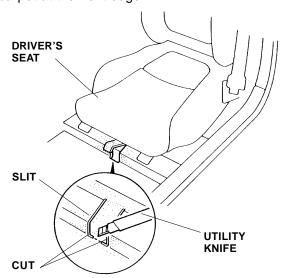
Using a utility knife, make an additional cut in the carpet between the two slits as shown.
