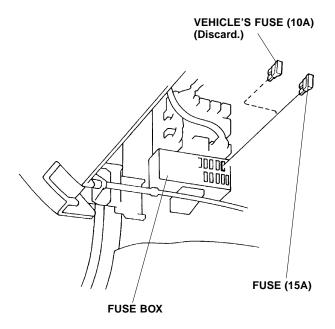
9. Attach the 15A fuse label to the back of the pocket over the existing 10A fuse label.
