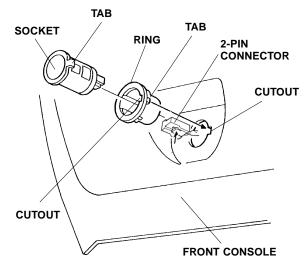
6. Connect the vehicle 2-pin connector to the socket of the cigarette lighter assembly, then push the socket into the ring while aligning the tab of the socket with the cutout of the ring.
