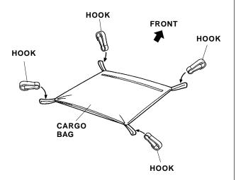
Attach the hooks to the anchors in the trunk.
