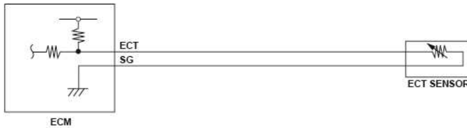
Fig. 13: Engine Coolant Temperature (ECT) Sensor Circuit Diagram
