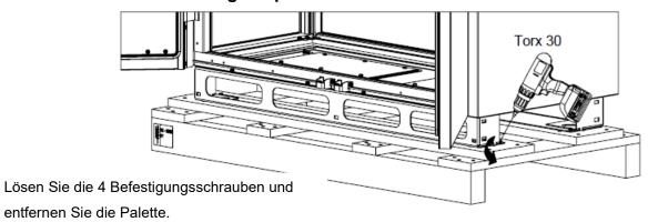
Undo the 4 fixing screws and remove the pallet.
