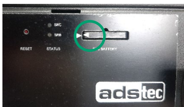
FIGURE 10: INSTALLING THE SRC4310 BACKUP BATTERY
