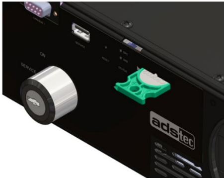
FIGURE 8: REMOVING THE SRC4310 BACKUP BATTERY
