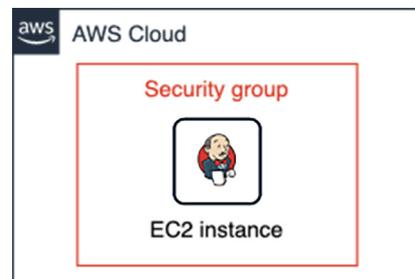
**Figure 3.10** The Jenkins standalone architecture on AWS consists of an EC2 instance behind a security group.
