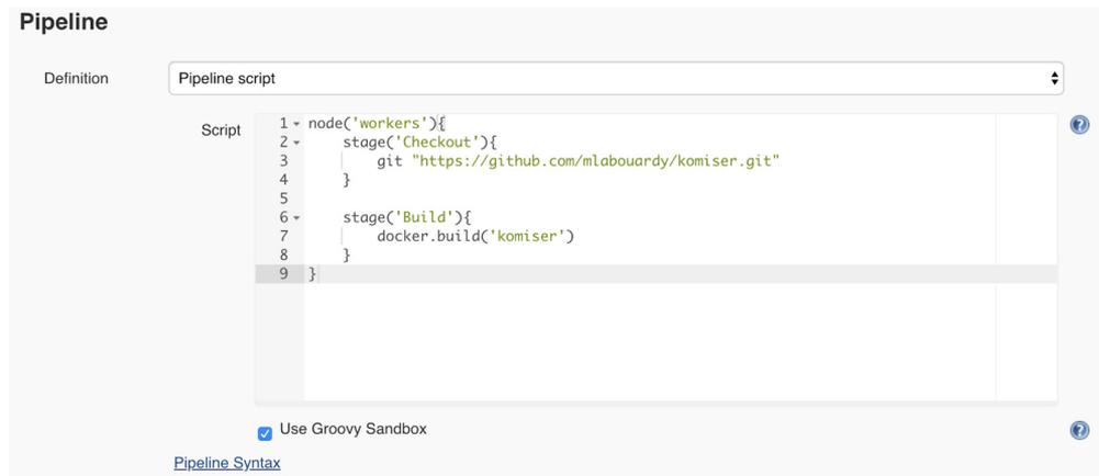
Figure 2.10 Using the stage keyword to define logical units
