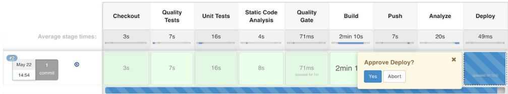
Figure 11.16 User approval for production deployment
