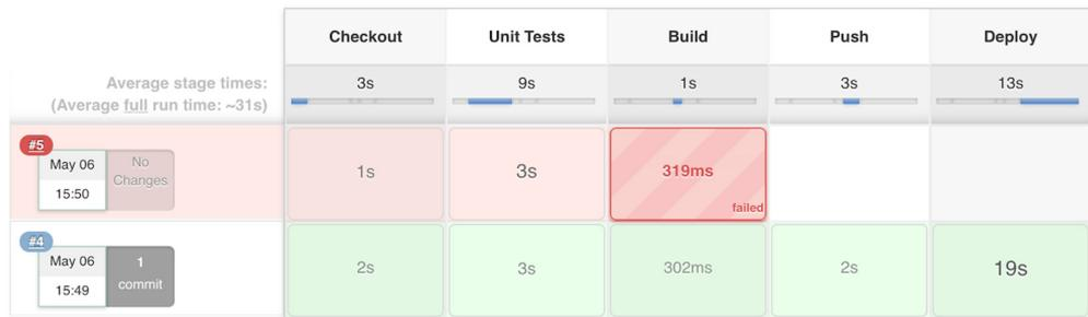
**Figure 10.34** Throwing an error within the Jenkins pipeline
