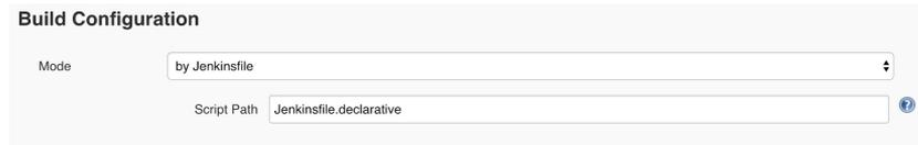
Figure 9.38 Jenkinsfile path configuration
