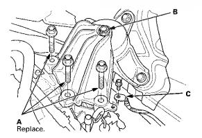
61. Remove the ground cable (C).
