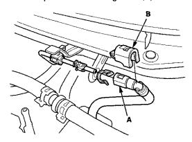
56. Connect the evaporative emission (EVAP) canister hose (A) and the brake booster vacuum hose (B).
