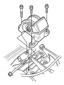
47. A/T model: Remove the rear engine mount (A), then remove the rear engine mount upper bracket (B).
