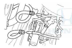
40. Disconnect the heater hoses (A) and the upper radiator hose (B).
