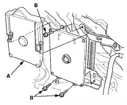
13. Disconnect the ECM/PCM connectors (A) and the engine wire harness connector (B).
