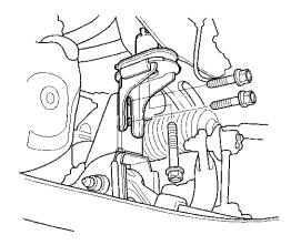
52. Attach the subframe adapter (VSB02C000016) to the subframe by looping the belt (A) over the front subframe (B), then secure the belt with its stop (C).
