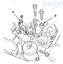
57. Remove the side engine mount bracket (B).
