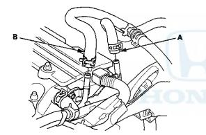
57. Connect the engine control module (ECM)/powertrain control module (PCM) connectors (A) and the engine wire harness connector (B).
