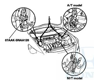
3. Attach the engine hanger adapter (VSB02C000015) to the threaded hole in the cylinder head.
