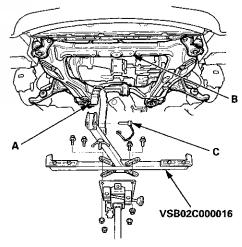
53. Raise the jack and line up the slots in the subframe adapter arms with the bolt holes on the jack base, then securely attach them with four bolts.
