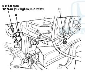
Install the A/C compressor (A), then connect the A/C compressor clutch connector (B).
