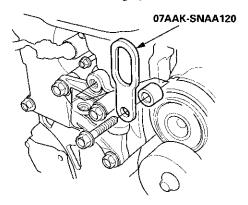
Install the side engine mount bracket (A), then tighten the new side engine mount bracket mounting bolts (B).
