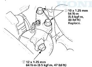
32. Loosen the mounting bolts for the upper transmission mount bracket, then retighten them to the specified torque.
