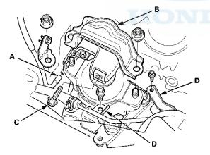
45. A/T model: Remove the ATF line brackets (D).
