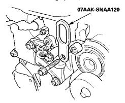
59. Attach a chain hoist (A) to the universal lifting eyelet (B) and the transmission hook (C), then lift the engine/ transmission until it is securely supported by the chain hoist, and remove the engine support hanger.
