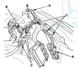
14. Remove the harness clamps (C) and the bracket (D).
