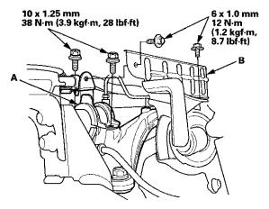
40. Install the P/S fluid line bracket (A), and secure the hose with the hose clamp (B).
