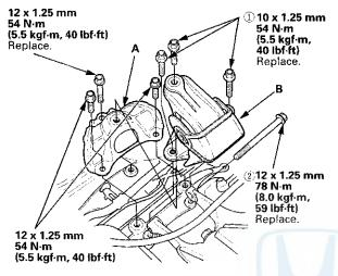
31. Loosen the mounting bolts for the side engine mount bracket, then retighten the bolts in the numbered sequence shown.
