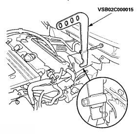
4. Install the engine support hanger (AAR-T1256), then attach the hook to the slotted hole in the engine hanger adapter. Tighten the wing nut (A) by hand to lift and support the engine/transmission.
