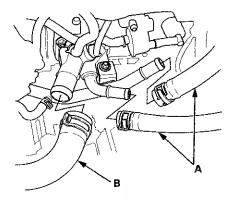
35. A/T model: Connect the ATF cooler hoses (A), and secure the hoses with the clips (B) (see page 14-220).
