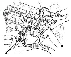
11. Disconnect the harness connector (B), and remove the harness connector from the bracket (C).
