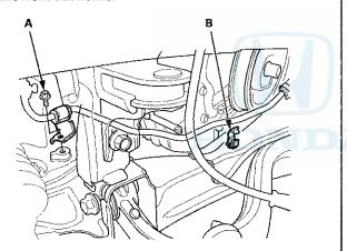
35. Remove the bolts securing the steering gearbox mounting bracket (A) and the heat shield (B), (right side)
