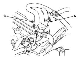
16. Remove the quick-connect fitting cover (A), then disconnect the fuel feed hose (B) (see page 11-314).
