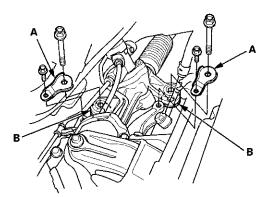
A/T model: Disconnect the automatic transmission fluid (ATF) cooler hoses, then plug the lines and hoses.
