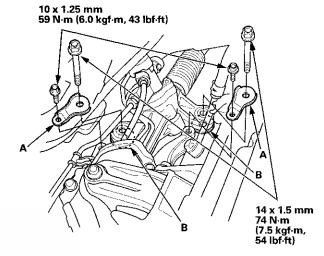
37. Install the two bolts (A) securing the power steering (P/S) fluid line brackets.
