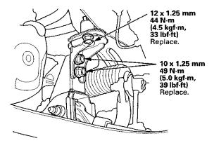
24. Tighten the nuts securing the lower transmission mount.
